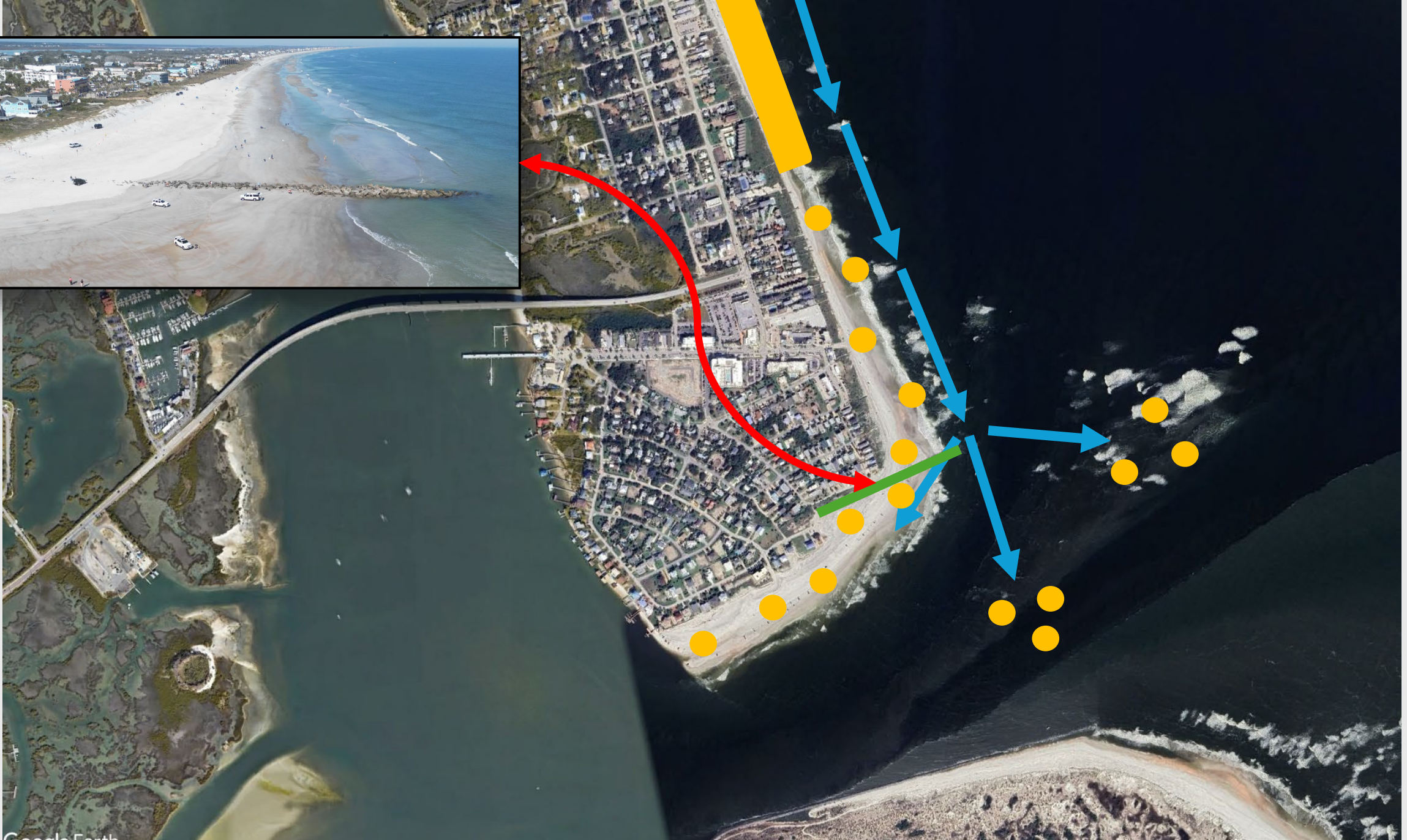
Current sediment movement passing through the jetty depositing in the inlet system and onto Porpoise Point
