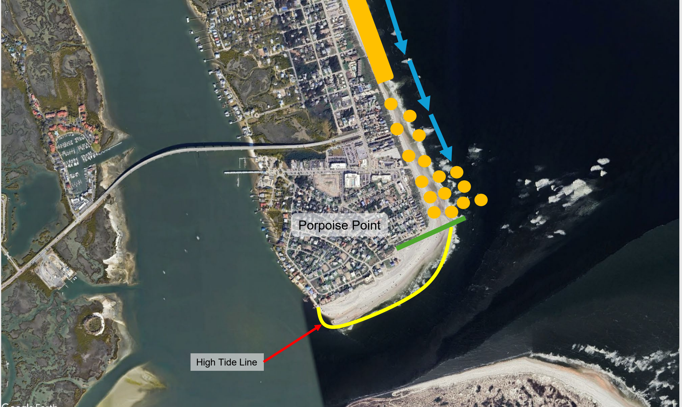
A properly functioning jetty would trap sand to the north building up the beach in Vilano
