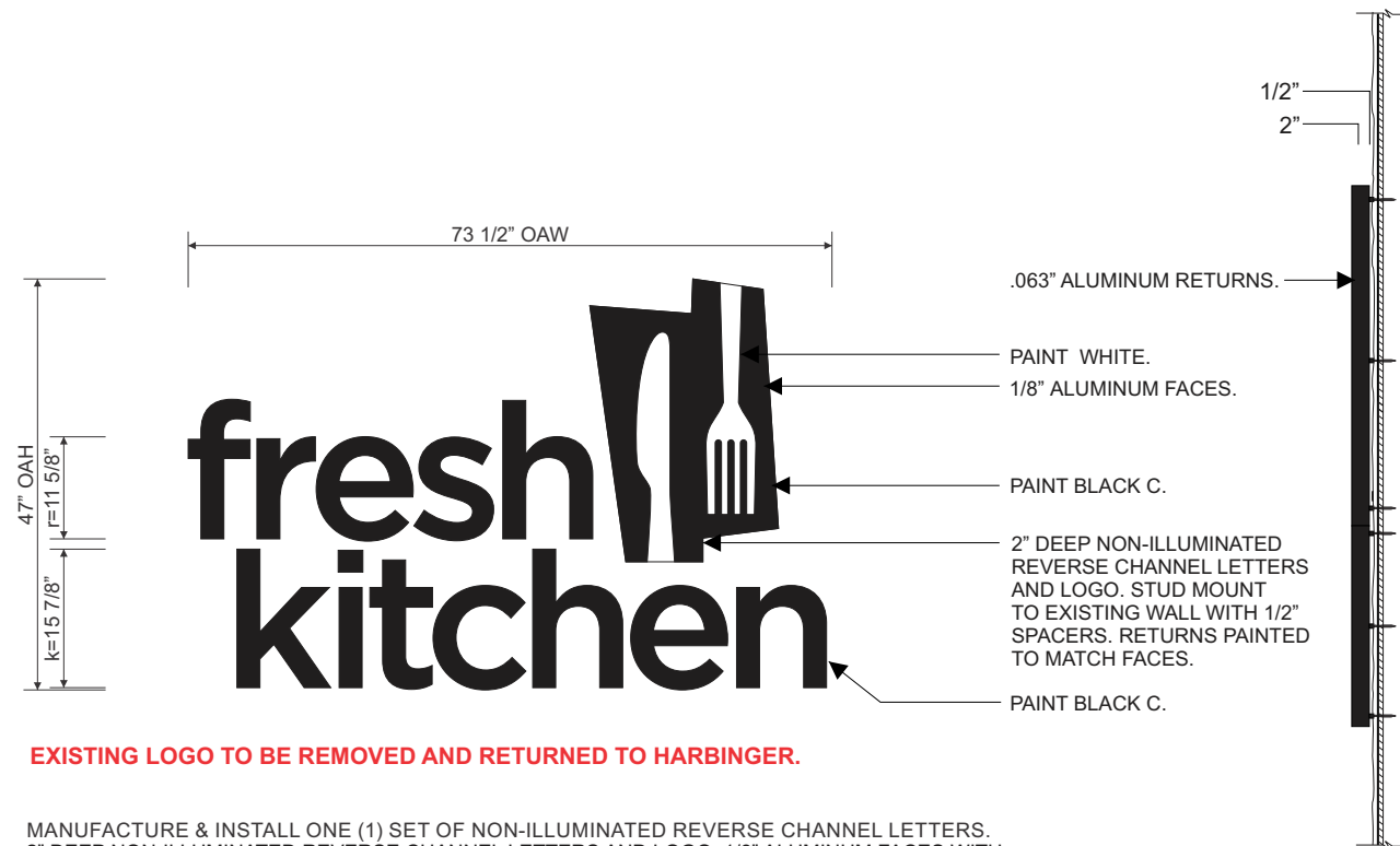
3 Front Elevation and End View - Non-Illuminated Reverse Channel Letters 1/2" = 1'-0"
