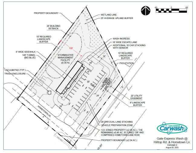
The above proposed site plan, provided by the applicant, depicts the layout of the car wash. The full Site Plan is included in **Attachment 1 Supporting Documents**.
